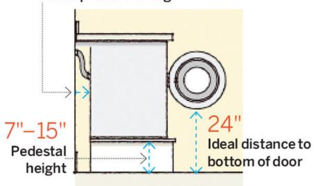
Laundry Room Numbers: Hookup Clearance The hookup clearance behind machines and pedestal height affect chore efficiency.
